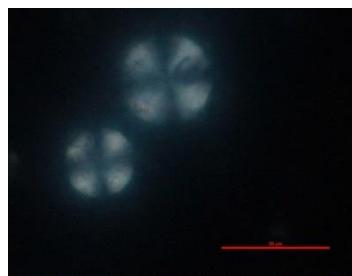
Fig.1. Maltese cross pattern from polarized light microscopy suggests presence of multilamellar vesicles in MON-DOPG mixtures
