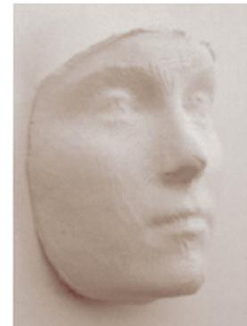
**Fig. 3** Physical model made by plaster moulding in stereolithography negative master.
